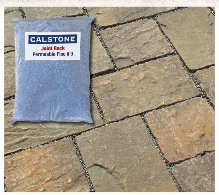
Until now the minimum joint width of permeable pavers was dictated by the largest particle sizes in locally available permeable joint fillers. ICPI recommends stone sizes 8, 89, or 9, for permeable joint fill. (bigger number = smaller stone) Calstone developed Fine #9 to meet the stone size # 9 standards with the smallest maximum stone size possible.
